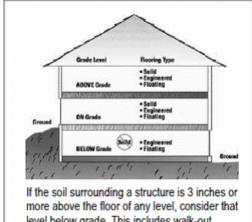
If the soil surrounding a structure is 3 inches of more above the floor of any level, consider that level below grade. This includes walk-out basements. In addition, the surrounding soil should be sloped away from the structure.
