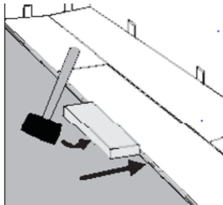
Step 5: Use hammer and tapping block to tap long edge of plank to ensure a tight fit. **ANY GAPPING CAN COMPROMISE THE LOCKING SYSTEM.**
