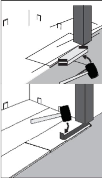
Step 1: Undercut space under door jamb to allow plank to slide freely. Tap long edge with hammer and tapping block too.
