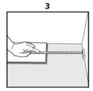
4. Start the second row with the leftover section of the previous row. The left- over section should measure at least 20cm (8"). Otherwise use a new plank and cut so that end joints are staggered properly with joints in the adjacent row.
