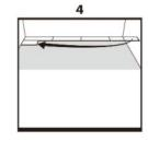
5. Place the floorboard at an angle against the floorboard in the previous row, press forward and fold down at the same time.
