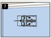
To adjust airflow, remove **plate** and bend dampers. For optimal air flow, push dampers past 90°.
