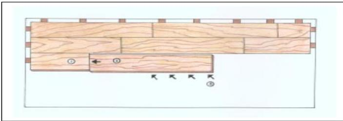
9. Last row: The minimum width of the last row (and first row) is 2" (50mm). Ensure to make this accommodation before installation begins. Minimum distance to keep away from end wall is 3/8" (10mm). Cut the planks lengthwise to fit.
