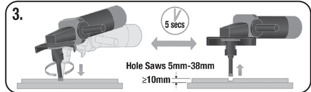
The QEP® Diamond Hole Saws for standard grinders are up to 50% faster and last up to 12X longer than standard diamond drill bits. They are designed for the easy, fast and accurate cutting of porcelain, ceramic and glass tiles. 1/4" and 5/16" sizes are integrated with an interior wax lubricant which melts while dry drilling and cools the cutting surface. For all sizes, water can be used as additional cooling to prolong the life of the bit.
