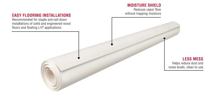
Silicone Vapor Shield is a moisture barrier underlayment made of 6 mil. wet strength paper with a backed silicone coating that will not allow moisture to penetrate through to the flooring planks.
