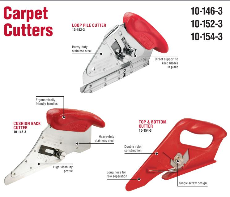
The ROBERTS Carpet Cutter assortment allows users to cut most carpet quickly and efficiently. These cutters feature 2-blade slots for cutting close to the pile's edge (10-152-3 and 10-146-3) or cutting either the top or bottom of the carpet (10-154-3). Knurled screws enable a fast, tool-free blade change. While these cutters are expertly designed for carpet installation, they can also be used for carpet removal.
