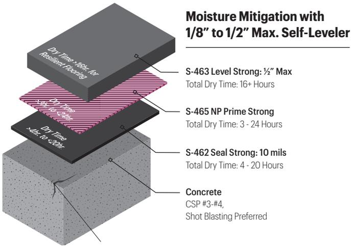
Use S-466 Patch Strong for repairing damaged areas that exceed CSP #6 Dormant hairline cracks of up to 1/32" can be covered with S-462 Seal Strong. Dormant joints and dormant cracks greater than 1/32" that will not be honored must be pre-filled with a highly fluid 100% rigid-drying crack filling material such as Ardex ArdFix™ intended for this purpose.
