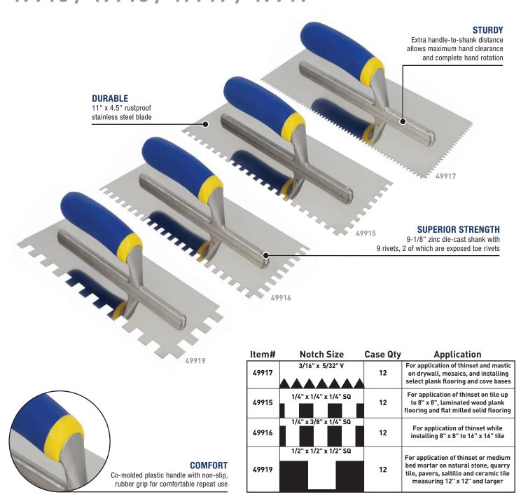
The QEP® Comfort Grip Stainless Steel Trowels are crafted with high quality materials for an extended life. With a rustproof, 11" x 4.5" blade, these trowel are great for professional installations and multi-use, DIY renovation projects. They feature 9 rivets, two of which are reinforced for durability, reducing the chances of trowel breakage, even in the most challenging installations.
