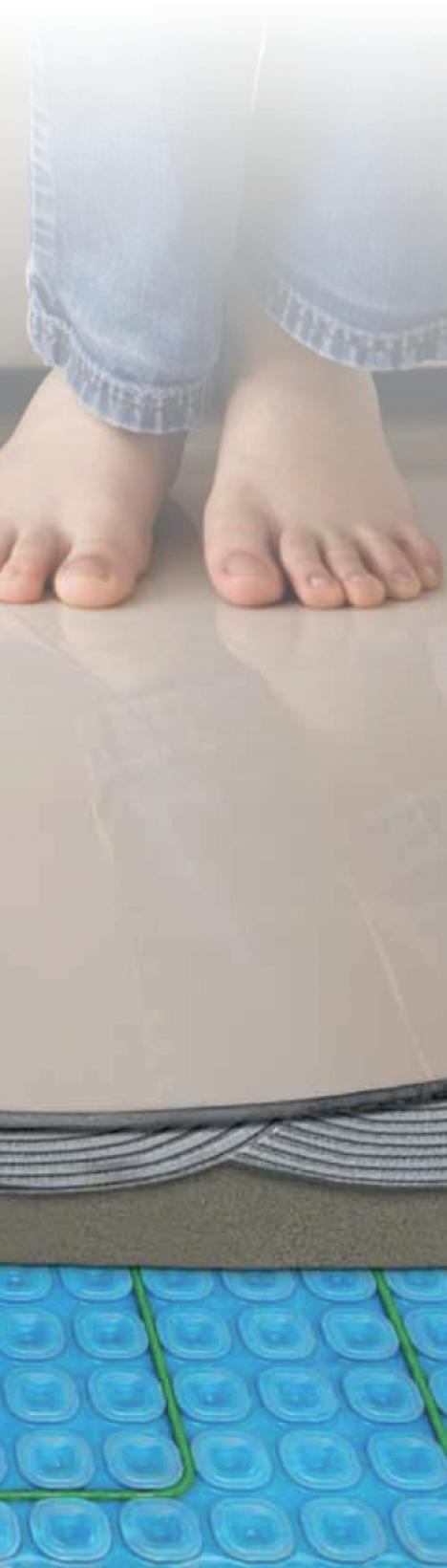
The patented **FLEXDECO uncoupling membrane** combines the benefits of an underlayment membrane with the comfort and convenience of electrical floor heating. The FLEXDECO uncoupling membrane can be installed over the entire subfloor as an uncoupling, crack isolating membrane. FLEXDECO's Cable is then installed in the areas where heat is desired. Once the FLEXDECO's Cable is installed you can begin tiling immediately, no waiting is necessary.
