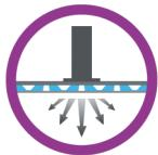
The FLEXDECO membrane's design allows loads to be evenly distributed from the tile covering to the subfloor. Each rounded square stud has a central cavity shaped like an inverted pyramid. When filled with mortar this inverted pyramid becomes an incompressible structure. These cavities act like pillars in a building support structure.
