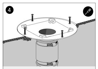
Firmly push the waste into position and screw the stainless steel screws into the shower base. Remove any excess caulk.
