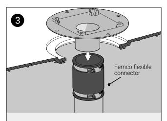
Connect the waste drain outlet pipe to the waste and test for any leaks before the next step.
