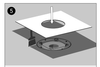
Cover the waste area in layer of waterproofing and firmly apply the gasket to the shower base and waste drain area.
