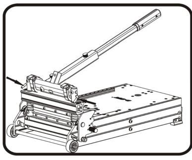
**Lock the Cutting Head**Use the provided Lock Pin to tuck the hole on the main column as shown. Make sure the cutting blade is in a close position when the cutter is not in use.
