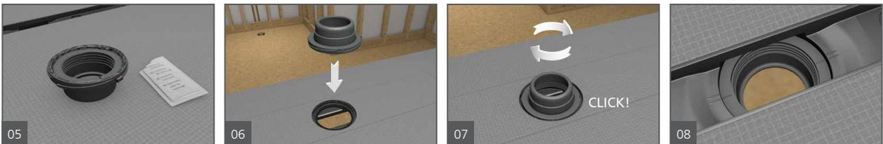
5. Apply the wedi provided safe Lubricant to the black rubber ring inside the wedi Drain Body.
