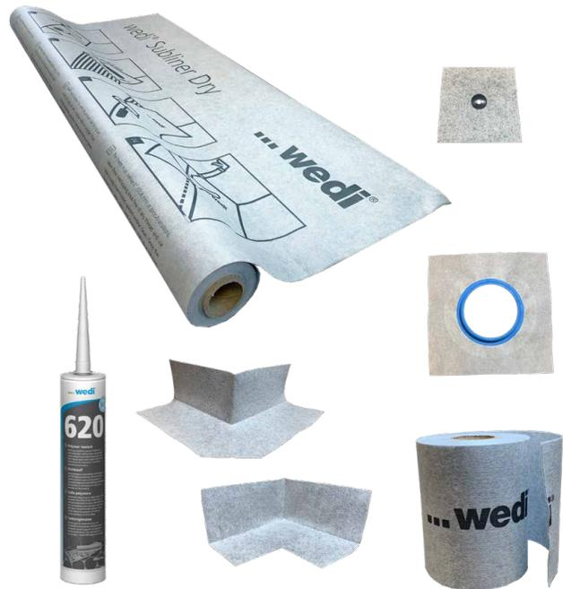
We also have special sealing tape options available for you, such as our tub sealing tape. wedi Tub Sealing Tape is equipped with a Butyl based adhesive strip which attaches to a plastic tub unit's perimeter outside edge before it's attached up onto blocking installed horizontally between framing studs. Here it creates a waterproofing back-up to a tub's traditional surround wall backers, which are prone to separate and leak at the transition from tub to wall.
