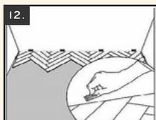
**Step 13** - Start each subsequent row by installing the A-panels from the left to the right and complete the row by laying the B-panels from the right to the left.
