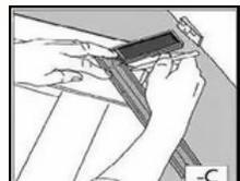
**Step 15** - Remove the spacers and cover the expansion gap with skirting boards or beadings.
