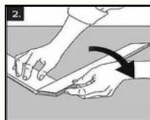
**Step 3** - Next panel is an A-panel. Again, press the long side of the new A-panel at an angle against the short side of the previous B-panel and fold down. Continue this process with as many panels that may fit along the starting wall.
