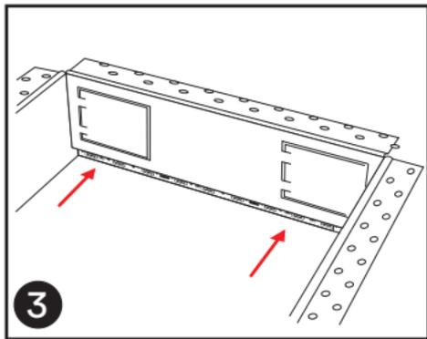
Use adhesive to secure the LED strip to the roof of the channel.
