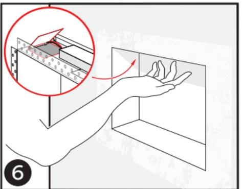
Maintenance post installation can be done through the concealed hinge doors.
