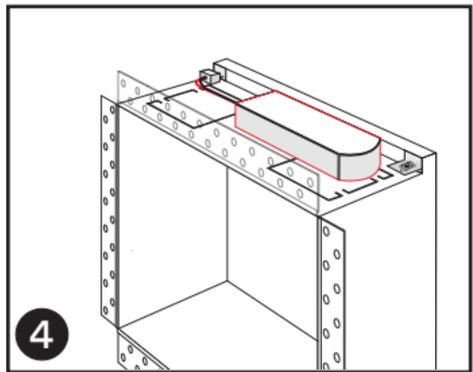
Connect the solderless clamp to the LED Strip, and attach the converter.
