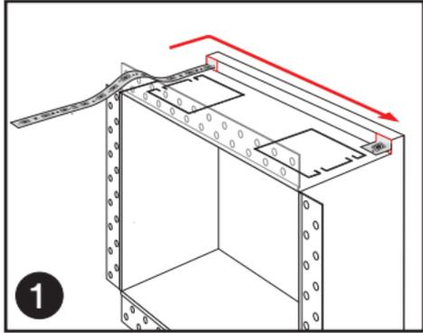
Line LED light strip along the inner top channel. Strip should not exceed channel width of  $\frac{1}{2}$  inch.
