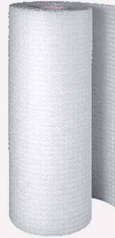
The Next Generation Uncoupling Mat for use under residential and commercial ceramic tile and stone installations, replacing traditional underlayment materials. Enhances the mechanical bond of adhesive mortar for faster drying and shorter wait times for grouting. Available in the standard STRATA\_MAT™ 1/8" (3 mm) version and STRATA\_MAT XT 5/16" (8 mm) thickness. Use STRATA\_MAT XT when installing typical 1/4" to 3/8" (6 to 9 mm) thick tile adjacent to 3/4" (19 mm) hardwood flooring.
