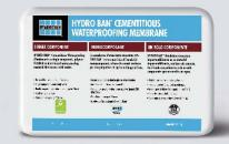
A one component, polymer fortified, cement based waterproofing material that mixes only with water. HYDRO BAN Cementitious Waterproofing Membrane handles negative and positive hydrostatic pressure up to 2 BARS (29 PSI) when applied at 40 mils (1 mm) thick. Flood test within 2 hours.
