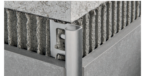
SATIN FINISH STAINLESS ST. AISI 304/1.4301-V2A with protective film bar length 2,7 lm - pack. 20 Pcs - 54 lm (H 4,5 mm - 108 lm) - 10/10 mm
