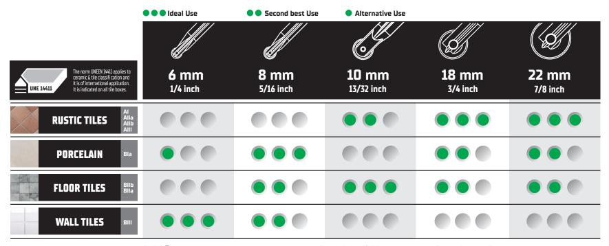
The RUBI® scoring wheels are manufactured using highly resistant, durable Tungsten Carbide. GDLD: Scoring wheel made from Tungsten Carbide with Titanium surface treatment, longlasting.
