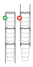
The chute chains should always be hanging down, never upwards.
