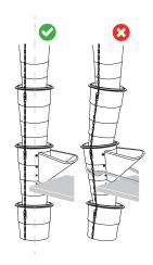
SIDE HOPPER DO NOT force onto the wall, making the column unbalanced. DO keep the column upright
