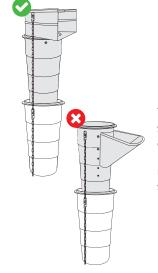
TOP HOPPER DO NOT start the column with a side hopper piece. Unsecured, loose or unscrewed hopper section
